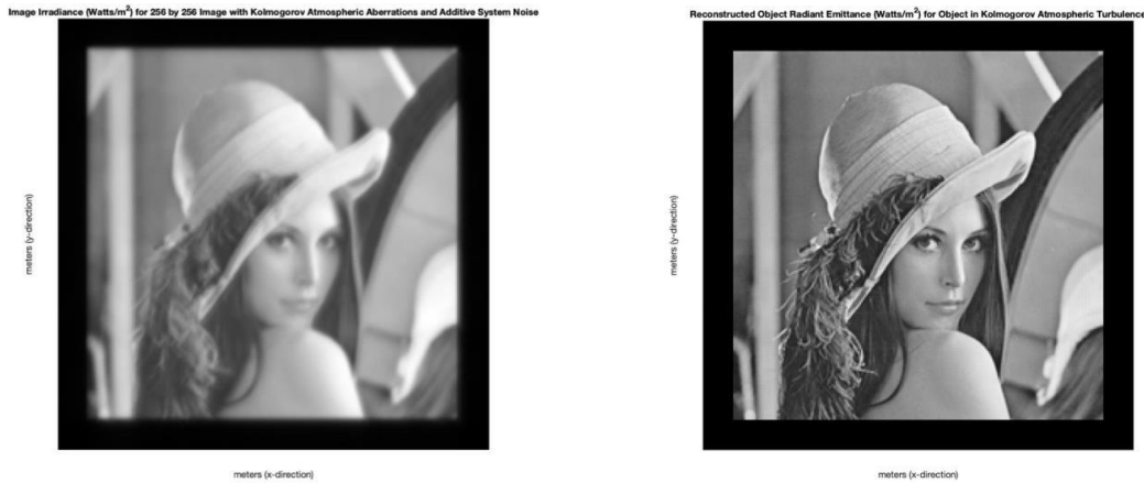
Figure 7 Aberrated image with Gaussian noise (left) and corrected image by using the WOLF method (right).
